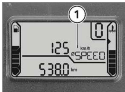
Average speed **1** is calculated on basis of the time elapsed since the last RESET. Times during which the engine was stopped are excluded from the calculation.
