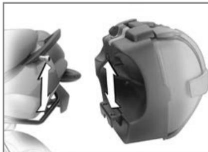
If a case wobbles or is difficult to fit, it has to be adapted to the gap between the top and bottom holders. The bottom bracket on the case can be moved up or down for this purpose.
